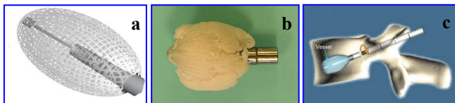
Fig. 1: (a) Vessel-X container (b) expanded by bone cement and (c) schematic diagram in the vertebrae
